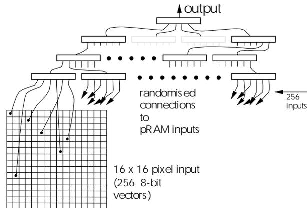
**Figure 3.** The pRAM neural network used in the position detection system.
